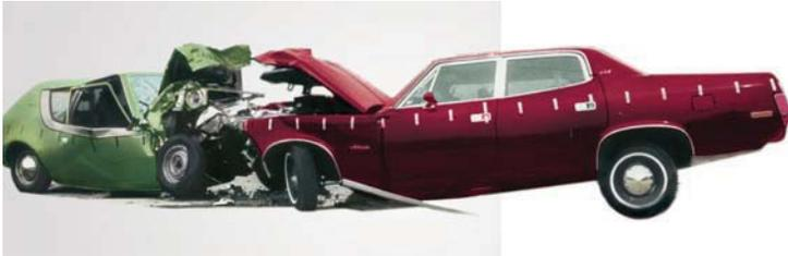
**CAR SIZE & WEIGHT, AGAIN:** The new series of crashes involving mini and midsize cars isn't the Institute's first foray into testing to demonstrate vehicle size and weight effects in frontal crashes. The first time was in 1971, and the test series featured an AMC Gremlin (above left) then known as an economy car, crashing into AMC's large Ambassador model.
