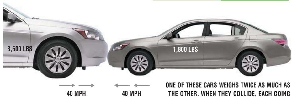
ONE OF THESE CARS WEIGHS TWICE AS MUCH AS THE OTHER. WHEN THEY COLLIDE, EACH GOING 40 MPH, THE HEAVY CAR PUSHES THE LIGHT ONE BACKWARD AT 13 MPH. THE VELOCITY CHANGE OF THE LIGHT CAR (53 MPH) IS TWICE THAT OF THE HEAVIER CAR (27 MPH).
